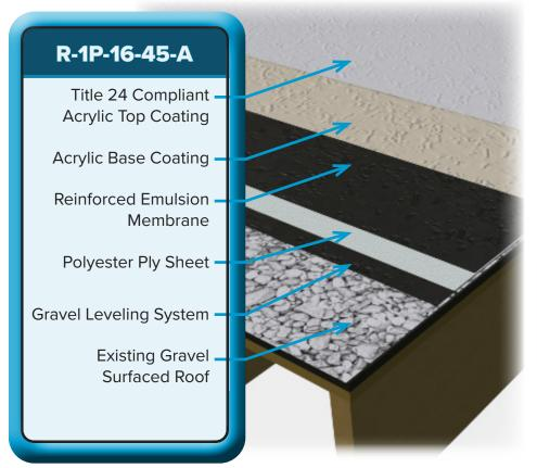
**WeatherWeld** R-1P-16-45-A is a completely seamless roof system designed for installation over existing gravel surfaced built-up-roofs.
